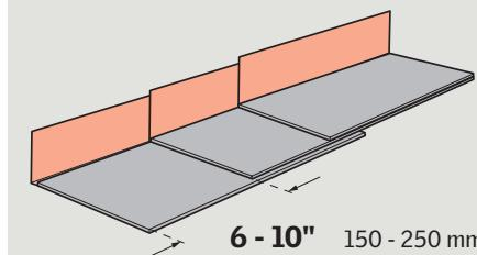
**ENGLISH:** For exposures between  $6$ " (150 mm) and  $10$ " (250 mm), use VELUX step flashing kit ZZZ 200 to replace the standard step flashing pieces and obtain adequate overlap.
