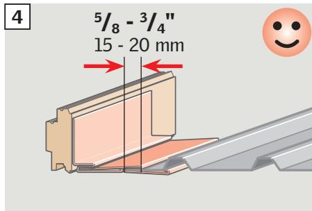
**ENGLISH:** When the roofing material conflicts with the retaining channel on the side flashing section, the auxiliary side flashing section must be used to extend the side flashing section.
