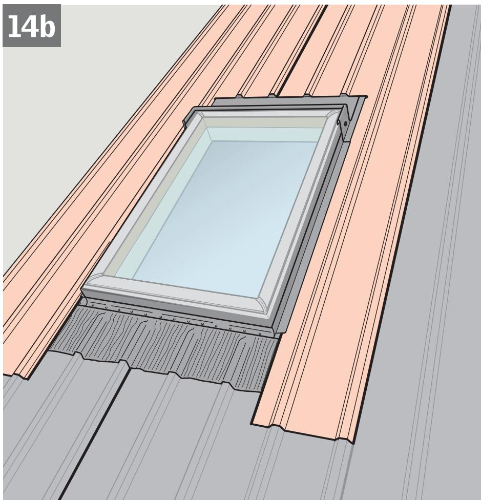
**ENGLISH:** With an installation including two or more roofing panels, the overlaps at the top can be avoided by cutting the side panels and add a notch to allow engagement on the sides.
