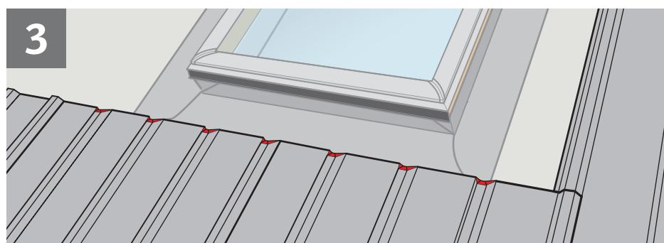
**ENGLISH:** Fold the edge of the roofing material for a smooth transition and to avoid sharp edges.
