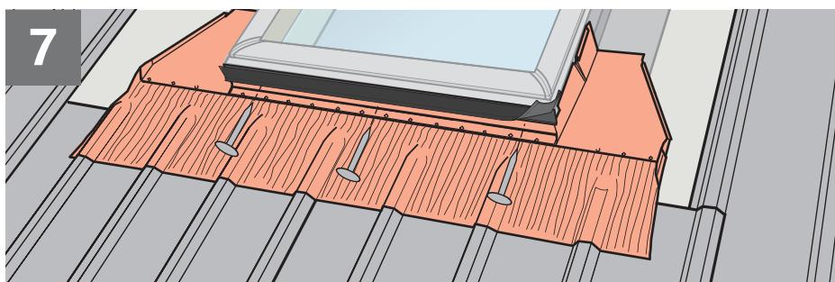
**ENGLISH:** Reposition sill flashing section and attach it to bottom frame with flashing nails provided.
