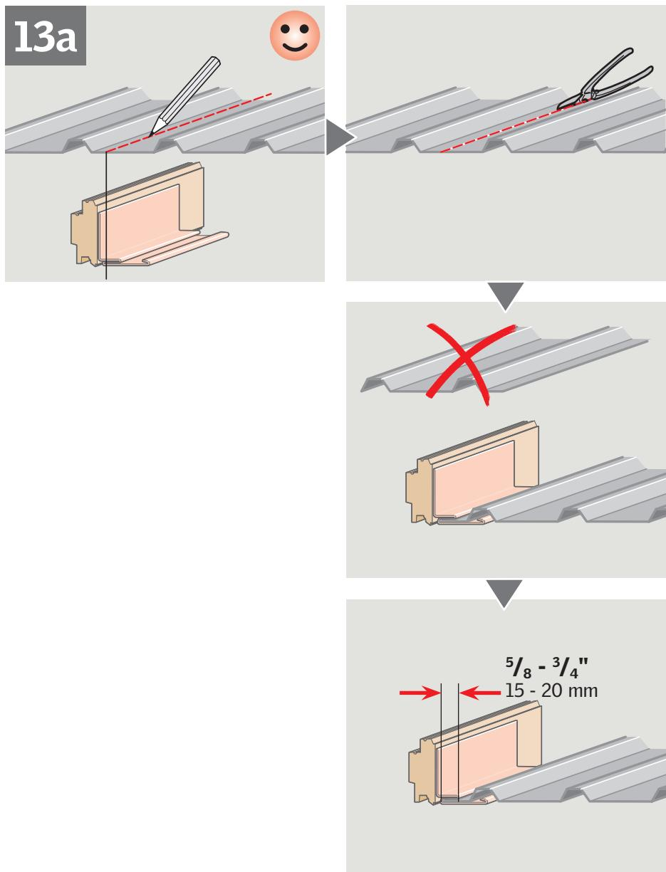
**ENGLISH:** When the roofing material fits into the retaining channel on the side flashing section, cut roofing material to engage with side flashing section as shown.
