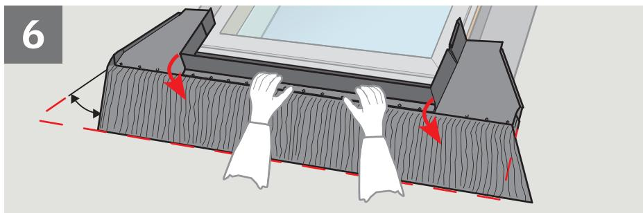
**ENGLISH:** Remove sill flashing section and bend the apron down as shown. This will ensure that the apron lies tightly against the roofing material.
