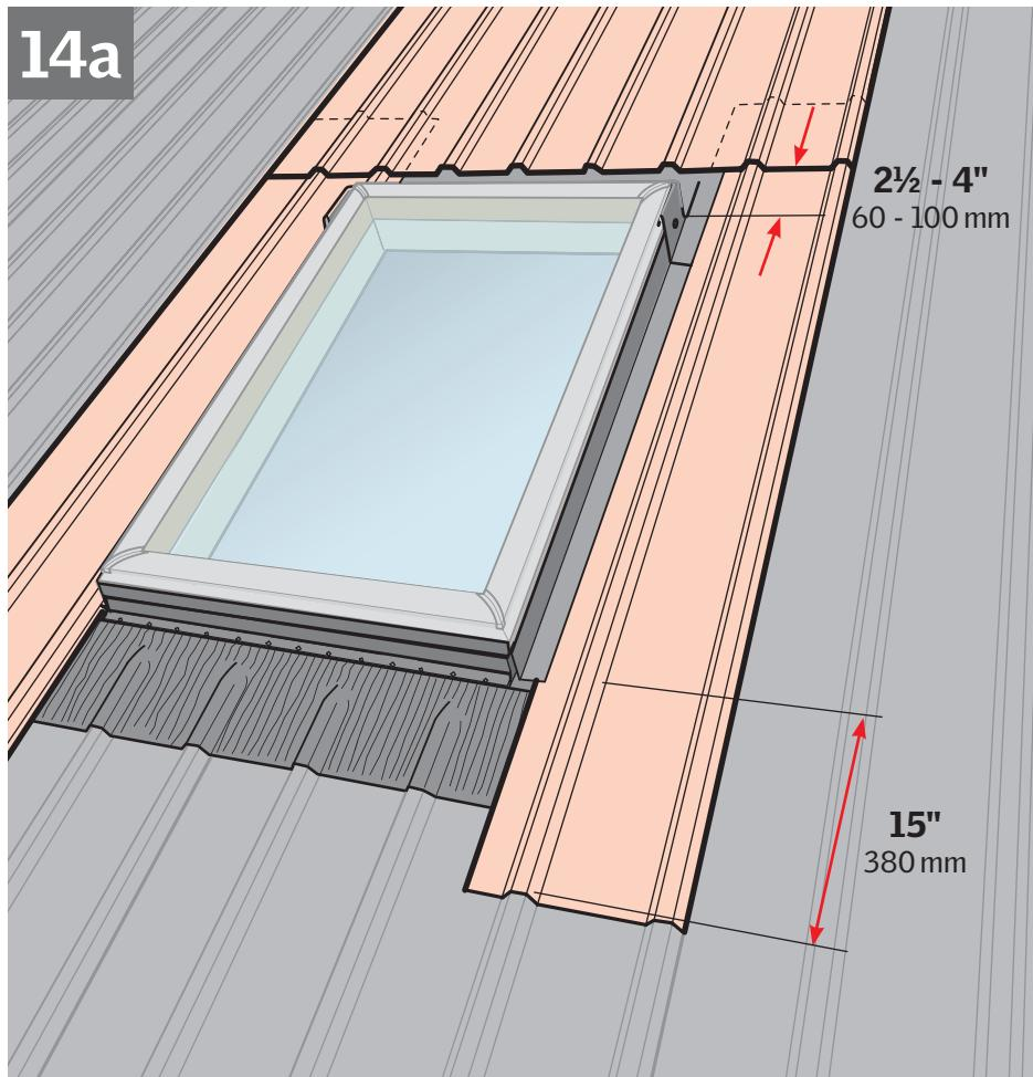
**ENGLISH:** Cut the roofing material maintaining 2½ - 4" (60 - 100 mm) clearance at the top. Make necessary overlaps and use closure strips between saddle flashing and roofing material, following roofing manufacturer's instructions. Do not perforate flashing when attaching the roofing material; maintain minimum distance for fasteners, see details.
