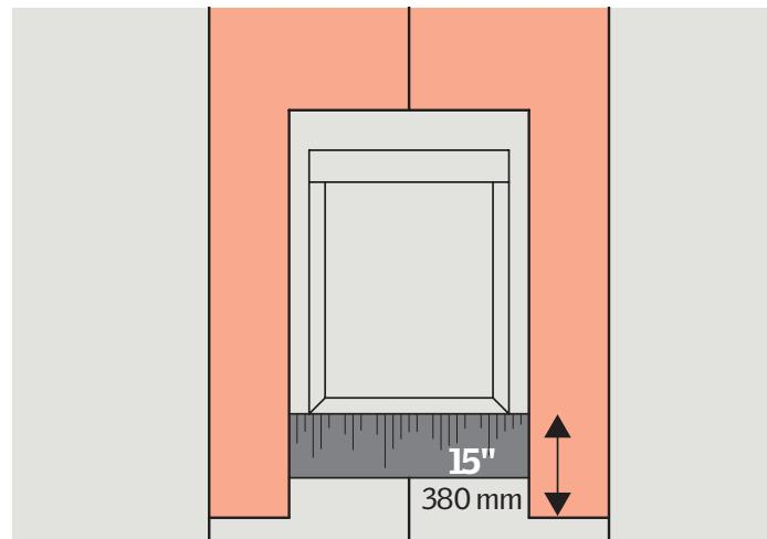
**ENGLISH:** EDM is designed for thin roofing materials (max thickness  $1\frac{1}{2}$  -  $1\frac{3}{4}$ " (38 - 45 mm)). Additional roofing material is always required to allow for necessary overlaps.
