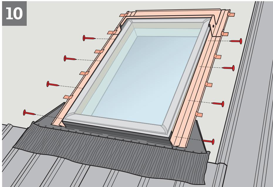
**ENGLISH:** Install and secure the side flashing sections and saddle flashing as shown.
