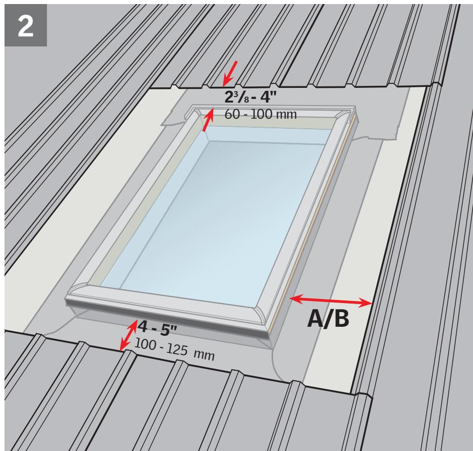
**ENGLISH:** Maintain illustrated clearances between frame and roofing material. If the skylight/roof window is located above a seam in the roofing material, the horizontal seam at the top can be avoided by removing all roofing material above the skylight/roof window.
