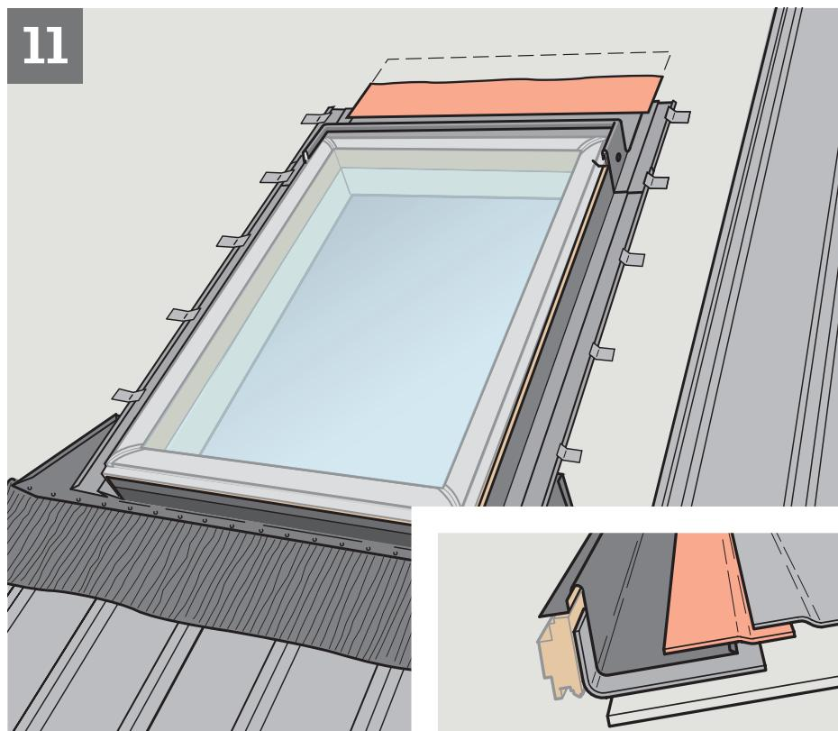
**ENGLISH:** Apply underlayment to allow drainage over the saddle flashing. Keep underlayment between retaining channels on side flashing sections.
