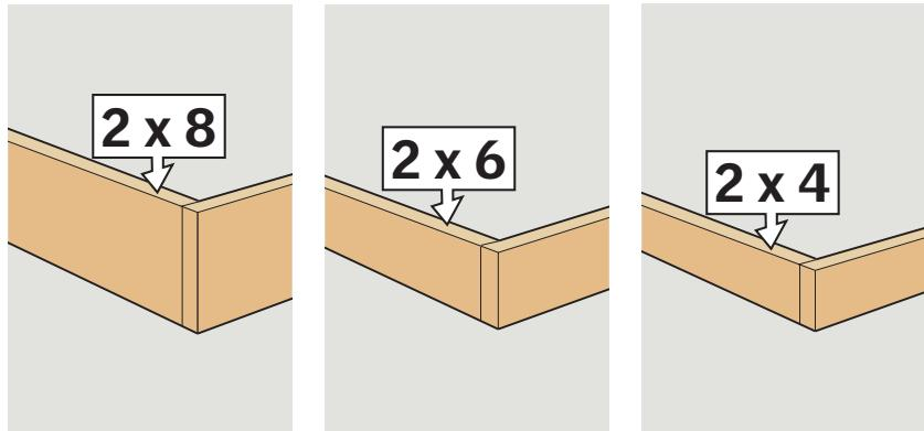
**ENGLISH:** Site-built curb to be provided by installer, with a height of 7 $\frac{1}{4}$ " (185 mm), 5 $\frac{1}{2}$ " (140 mm) or 3 $\frac{1}{2}$ " (90 mm).
