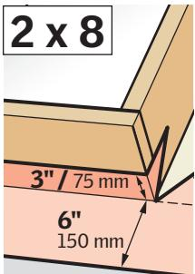
**ENGLISH:** Wrap the bottom and the corners of the skylight curb with the underlayment and create water-shedding laps over roofing underlayment.
