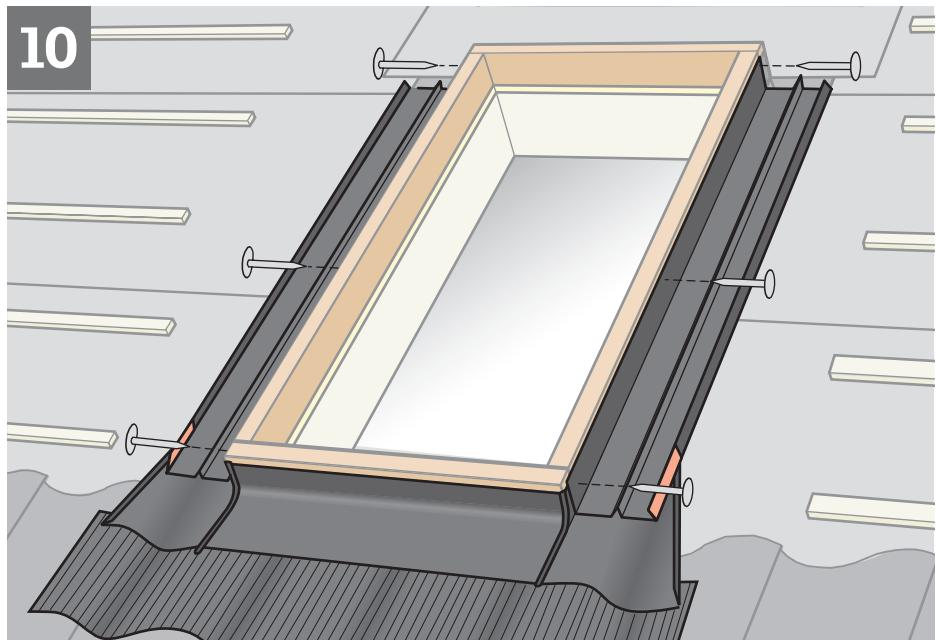
**ENGLISH:** Cut side sections to match size of curb. Modify side sections to allow for a smooth transition from sill flashing section to deck level and attach side sections to curb with roofing nails.
