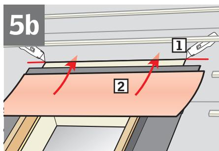
**ENGLISH:** Wrap the sides and the corners of the skylight curb with VELUX adhesive skylight underlayment and create water-shedding laps over roofing underlayment.
