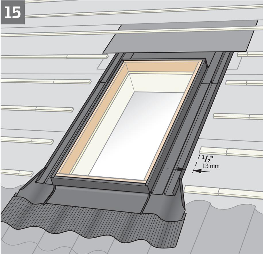
**ENGLISH:** Install roof battens as shown. Consider installing a tile support batten (not supplied) attached with wire straps at the top.
