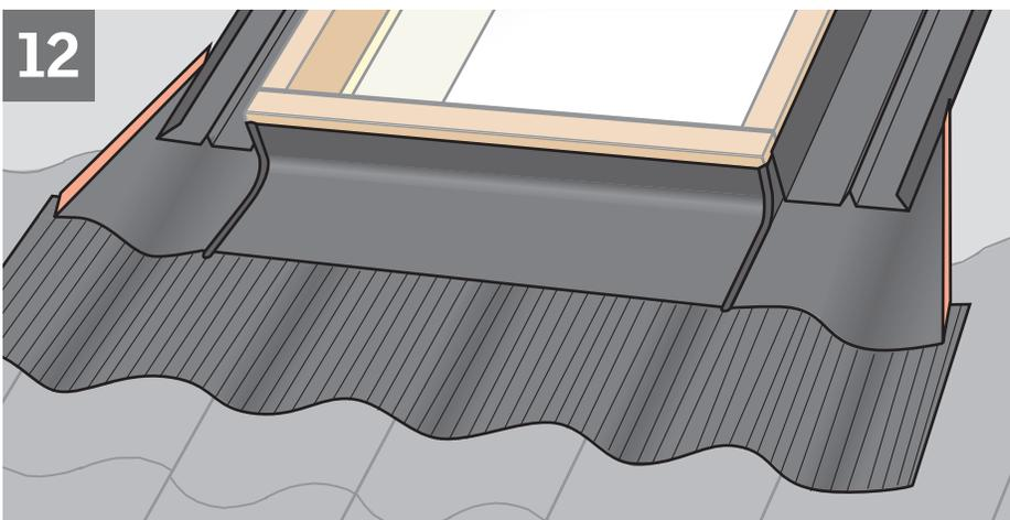
**ENGLISH:** Flatten down bottom edge of apron over roofing material as shown.
