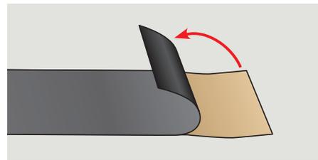
**ENGLISH:** To ensure waterproofing, skylight curbs shall be completely wrapped in VELUX adhesive skylight underlayment as indicated. Underlayment must be applied before installing the flashing.
