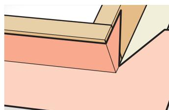
**ENGLISH:** Wrap the bottom and the corners of the skylight curb with the underlayment and create water-shedding laps over roofing underlayment.
