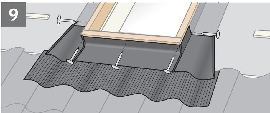
**ENGLISH:** Reposition sill flashing section and attach it to curb with roofing nails as shown.
