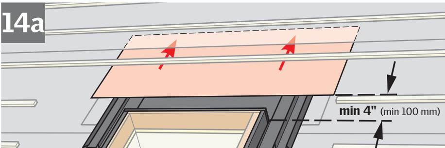
**ENGLISH:** To allow for proper drainage, interweave roofing underlayment as shown in **14a** for new construction applications. For retrofit applications, interweave roofing underlayment as shown in **14b**.
