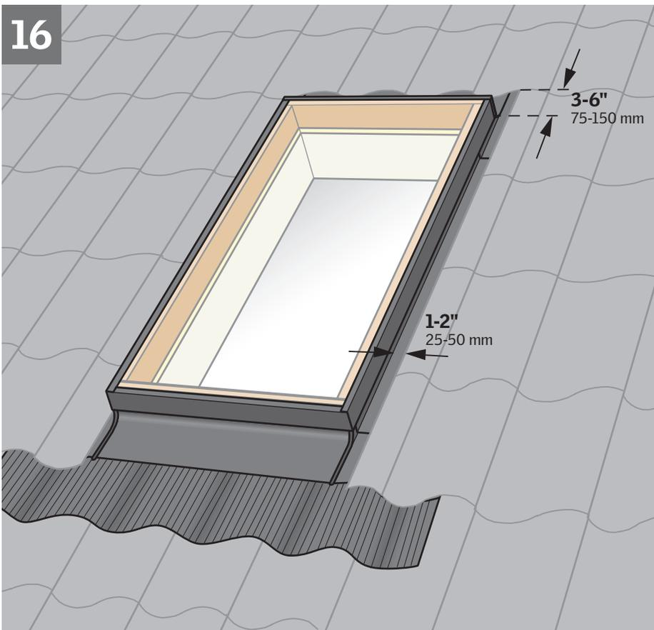
**ENGLISH:** Install roofing material. Observe distance to curb as shown.
