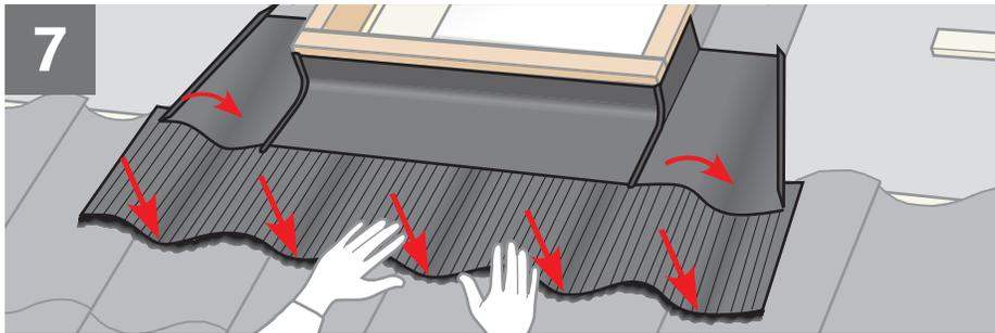
**ENGLISH:** Position sill flashing section and dress apron and side pieces over the roofing material.
