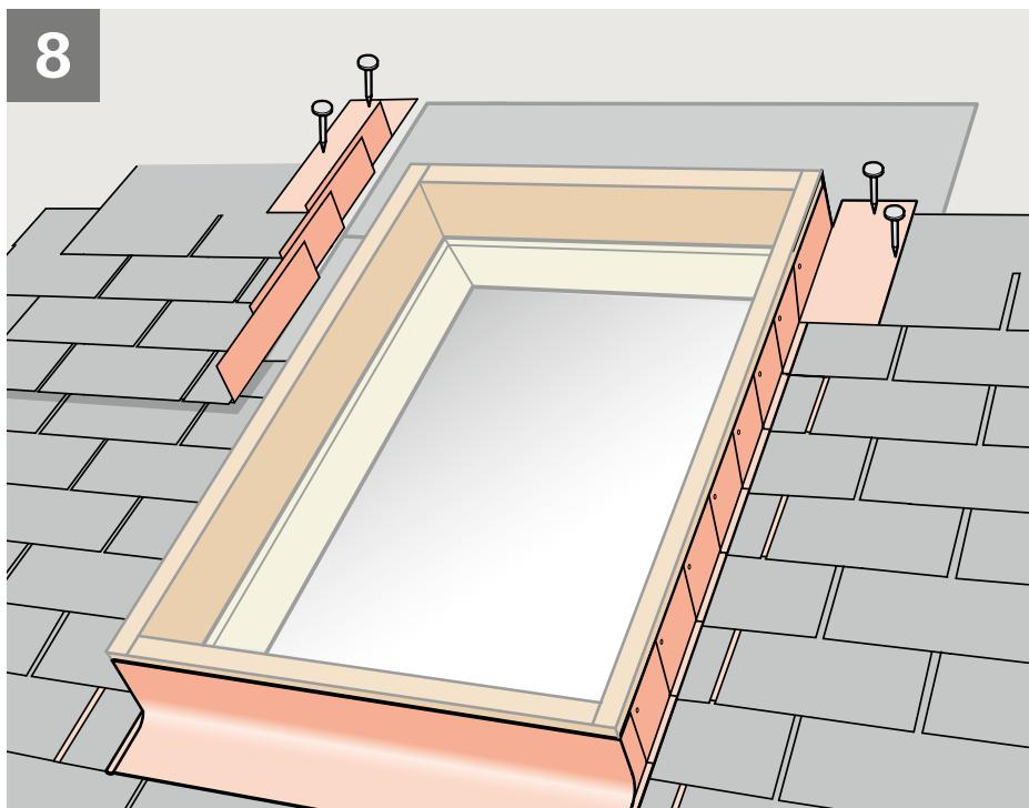
**ENGLISH:** Install step flashing pieces and roofing material.
