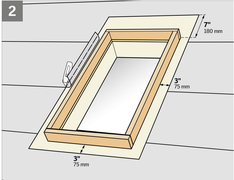
**ENGLISH:** To ensure waterproofing, skylight curbs shall be completely wrapped in VELUX adhesive skylight underlayment as indicated. Underlayment must be applied before installing the flashing. Remove existing roofing underlayment around the rough opening as shown.
