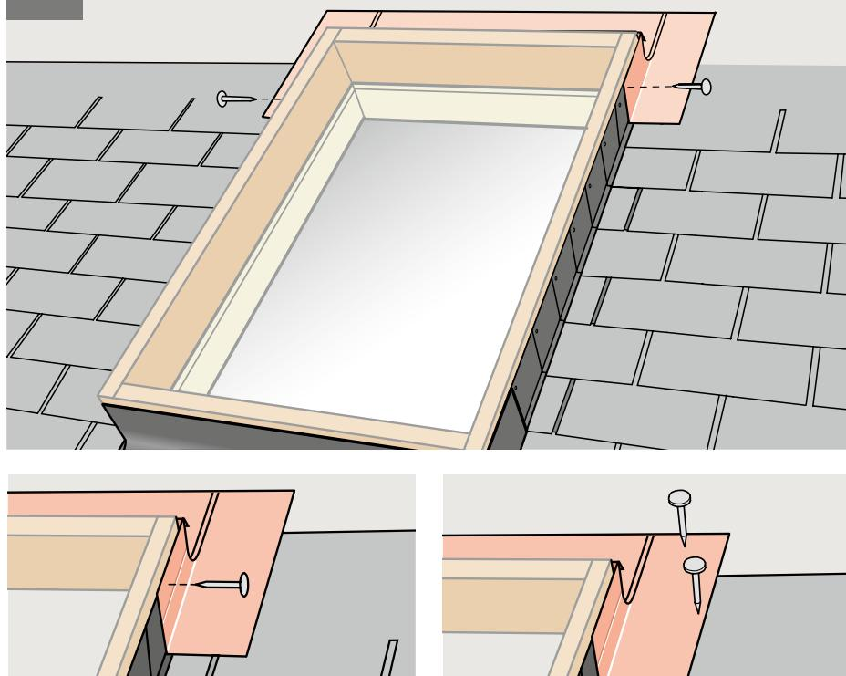
**ENGLISH:** Install and attach saddle flashing to curb or to roof with roofing nails as shown.
