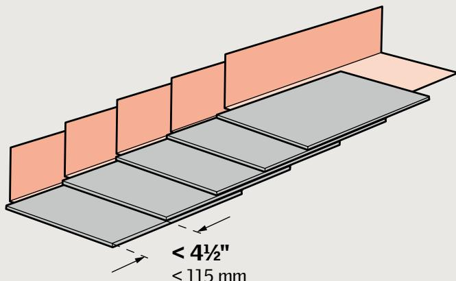
**ENGLISH:** For exposures less than  $4\frac{1}{2}$ " (115 mm) or greater than  $5\frac{1}{2}$ " (140 mm), a supplementary VELUX step flashing kit ZZZ 200 0000C may be required.
