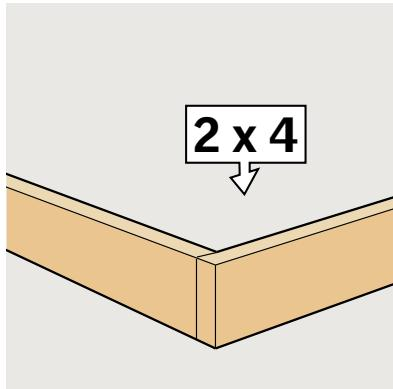
**ENGLISH:** Site-built curb to be provided by installer, with a height of  $5\frac{1}{2}$ " (140 mm) or  $3\frac{1}{2}$ " (90 mm).
