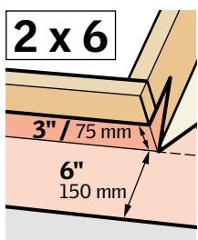
**ENGLISH:** Wrap the bottom and the corners of the skylight curb with the underlayment and create water-shedding laps over roofing underlayment.
