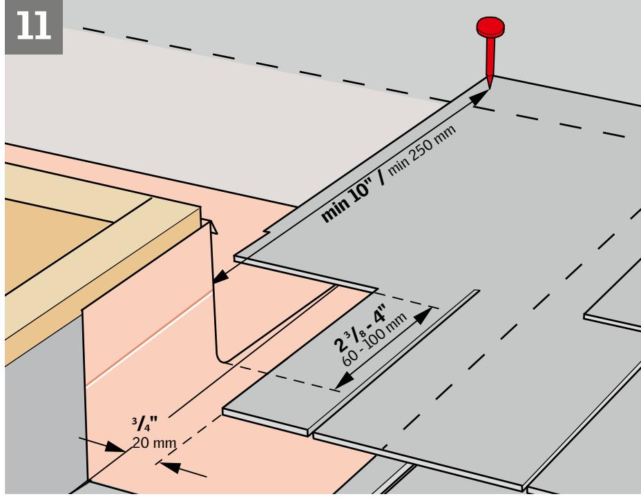
**ENGLISH:** Observe distance to roofing material. Do not nail through the saddle flashing when attaching the roofing material.
