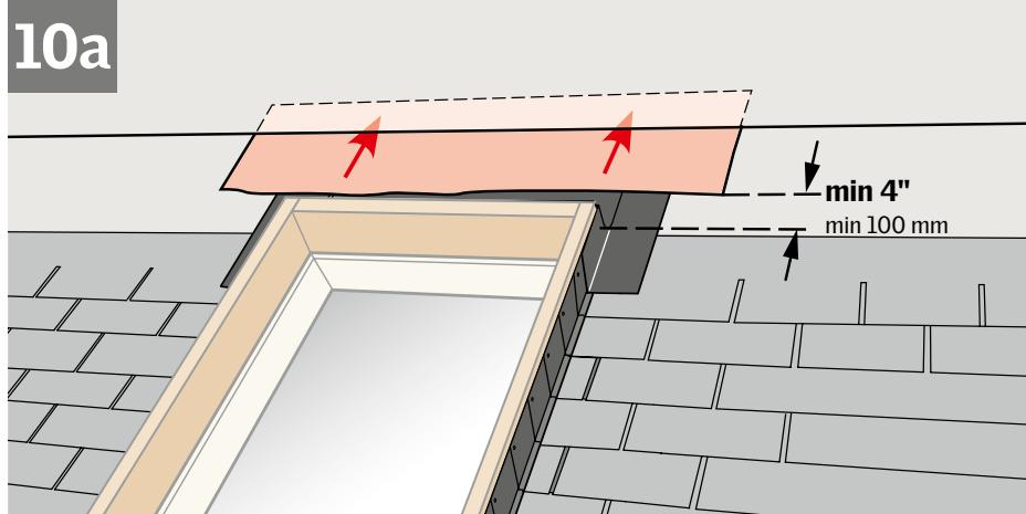
**ENGLISH:** To allow for proper drainage, interweave roofing underlayment as shown in **10a** for new construction applications. For retrofit applications, interweave roofing underlayment as shown in **10b**.
