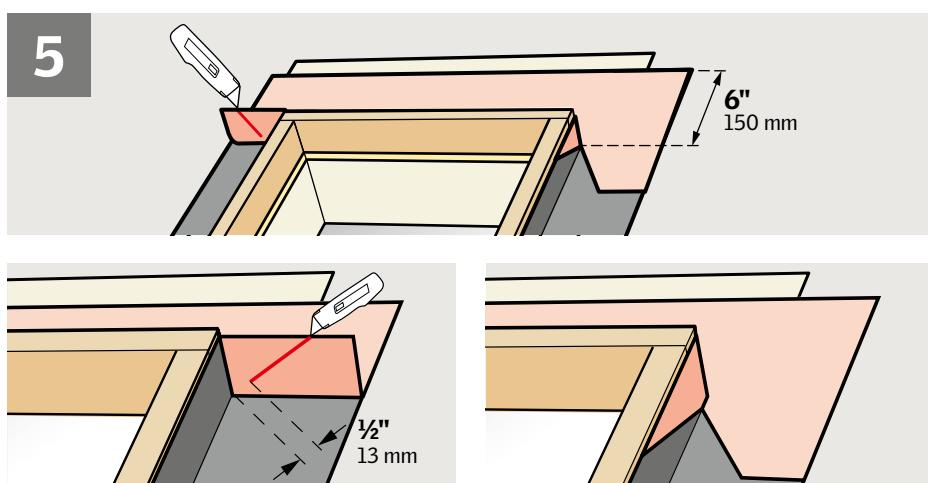
**ENGLISH:** Wrap the top and the corners of the skylight curb with VELUX adhesive skylight underlayment and create proper water-shedding lap.
