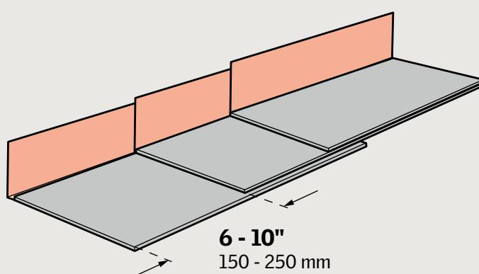
**ENGLISH:** For exposures between 6" (150 mm) and 10" (250 mm), use VELUX step flashing kit ZZZ 200 0000C to replace the standard step flashing pieces and obtain adequate overlap.
