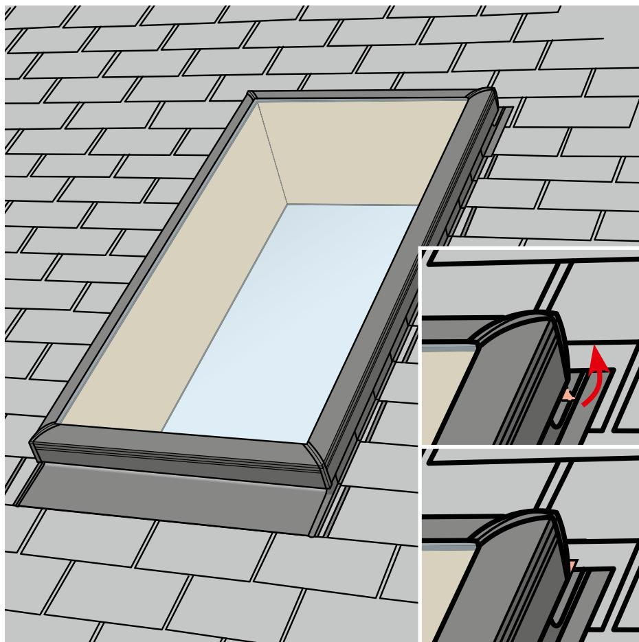
**ENGLISH:** When installing the skylight on a curb with a height of  $3\frac{1}{2}$ " (90 mm), bend the visible part of the saddle flashing as shown for extra protection.
