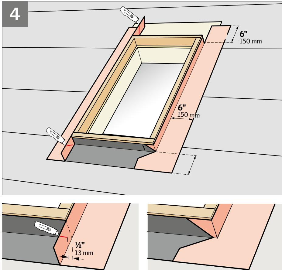
**ENGLISH:** Wrap the sides and the corners of the skylight curb with VELUX adhesive skylight underlayment and create water-shedding laps over roofing underlayment.
