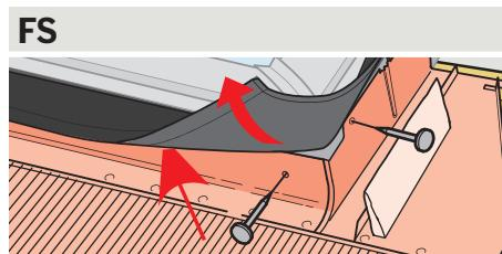
**ENGLISH:** Reposition sill flashing section and attach it to bottom frame with roofing nails provided.
