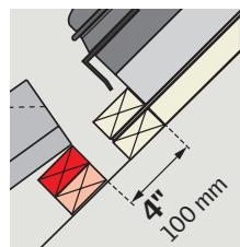
**ENGLISH:** If a full course of tiles below the skylight/roof window cannot be accomplished, the tiles at the bottom corners must be cut to leave a 6" (150 mm) clearance to the side frames. Install support battens as shown to compensate for the cut away part of the tiles and secure tiles.
