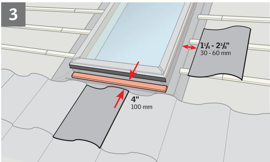
**ENGLISH:** Maintain illustrated clearances between frame and roofing material and install support batten for sill flashing section. This will ensure correct drainage of water from the sill flashing section.
