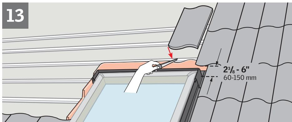
**ENGLISH:** Maintain distance to frame as shown; cut tiles, if necessary. Trim foam gasket to fit tiles. Adjust the tile support and bend strips to hold it in place **a**.
