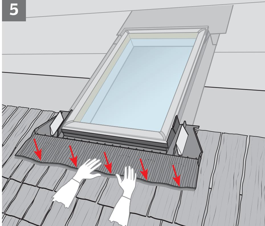
**ENGLISH:** Position sill flashing section and dress apron over the roofing material.
