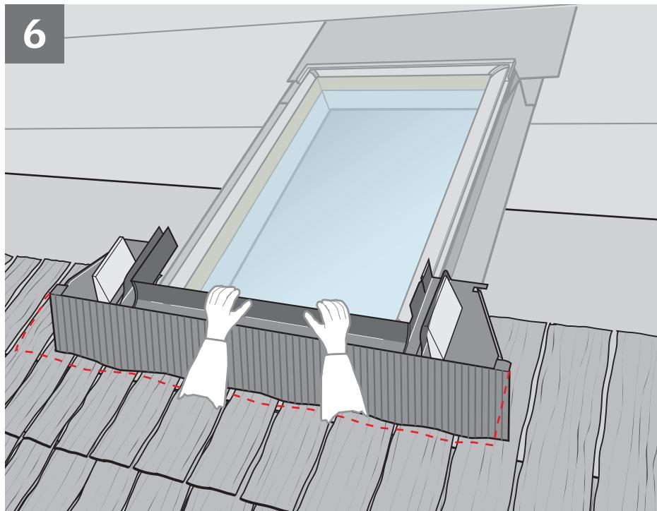
**ENGLISH:** Remove sill flashing section and bend the apron down as shown. This will ensure that the apron lies tightly against the roofing material.
