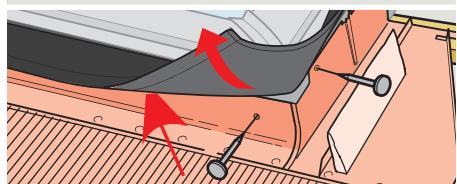
**ENGLISH:** Reposition sill flashing section and attach it to bottom frame with roofing nails provided.
