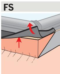
**ENGLISH:** When installing the first course of interlayer reaching the skylight/roof window, wrap this course around the bottom frame.
