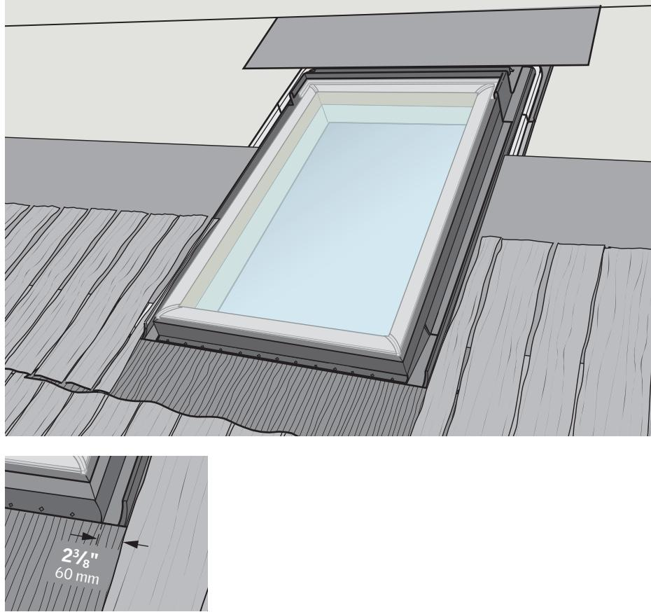
**ENGLISH:** Complete installation of cedar shingles and interlayment. Maintain distance to frame as shown.
