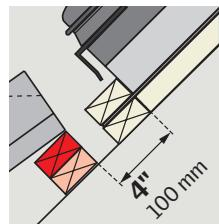
**ENGLISH:** If a full course of tiles below the skylight/roof window cannot be accomplished, the tiles at the bottom corners must be cut to leave a 6" (150 mm) clearance to the side frames. Install support battens as shown to compensate for the cut away part of the tiles and secure tiles.
