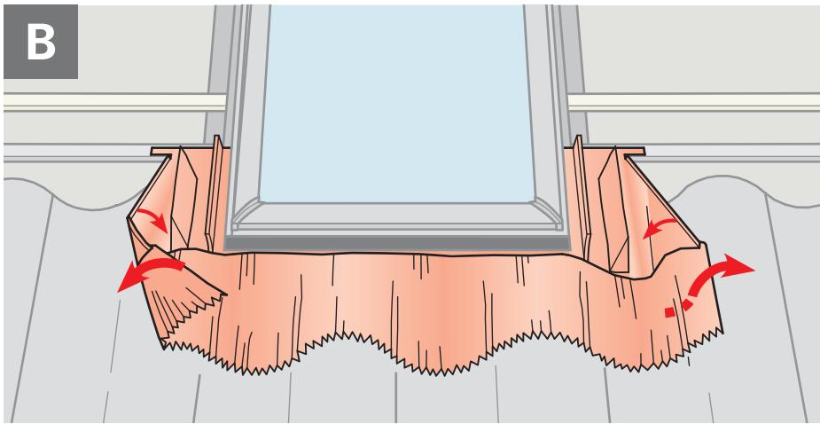
**ENGLISH:** In case of cut corner tiles, bend side pieces over the roofing material.
