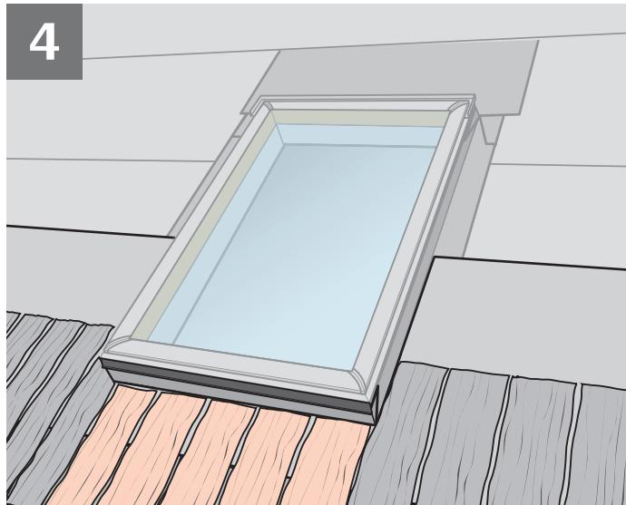
**ENGLISH:** Install a course of cut cedar shakes below the skylight/roof window. Maintain distance to frame as shown.
