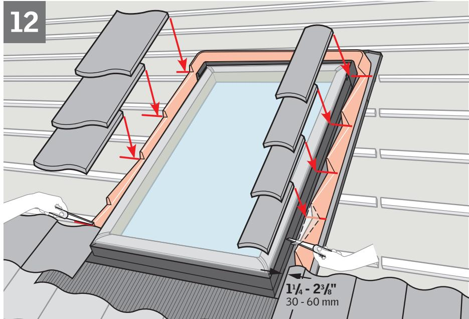
**ENGLISH:** Install tiles and maintain distance to frame as shown; cut tiles, if necessary. Trim and cut foam gasket for optimum contact to roofing material.
