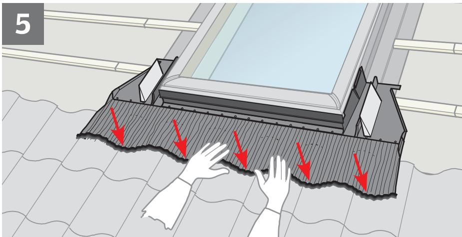
**ENGLISH:** Position sill flashing section and dress apron over the roofing material.
