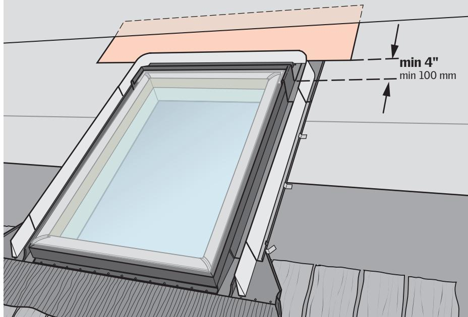
**ENGLISH:** To allow for proper drainage, interweave roofing underlayment as shown.
