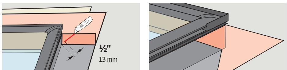
**ENGLISH:** To allow for proper drainage, interweave VELUX adhesive skylight underlayment as shown in **9a** for new construction applications. For retrofit applications, interweave VELUX adhesive skylight underlayment as shown in **9b**.
