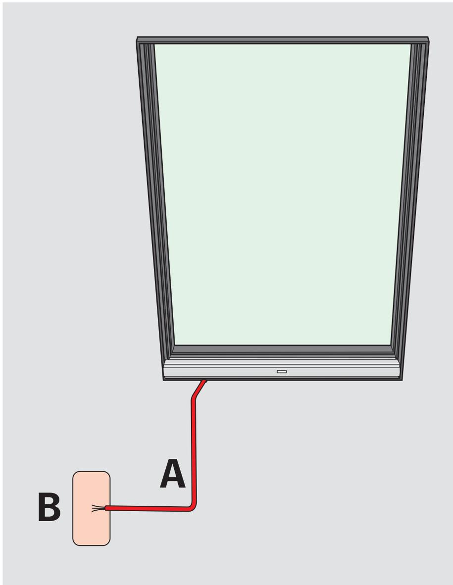
**ENGLISH:** A junction box or an outlet box (not provided with skylight) is required for permanent connection of the 20 ft (6 m) skylight power cable. A single phase 120 V, 60 Hz, 40 W branch circuit (continuous electrical feed) is required. The branch circuit must be protected by a 15 A circuit breaker or time delay fuse.
