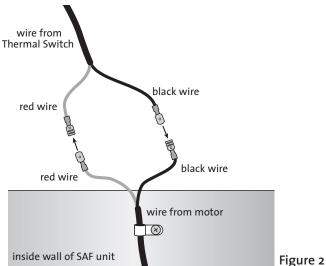
The **Thermal Snap Switch** is designed to turn on the Natural Light Solar Attic Fan (SAF) when the temperature in the attic reaches approximately 80° F. It will turn off the motor when the temperature in the attic reaches 70° F.
