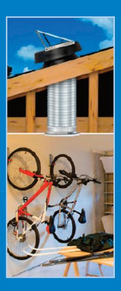
The Garage Exhaust Vent is an add-on kit that converts all Natural Light roof and curb mounted Solar Attic Fans into a garage ventilation system. An adapter sleeve is attached to the underside of the fan assembly and connected to a flexible duct pipe that runs through the attic. The kit includes an attractive white powder-coated ceiling vent that attaches to the garage ceiling. The systems venting capacity will depend on the model size of the solar attic fan and the length of flexible pipe used.
